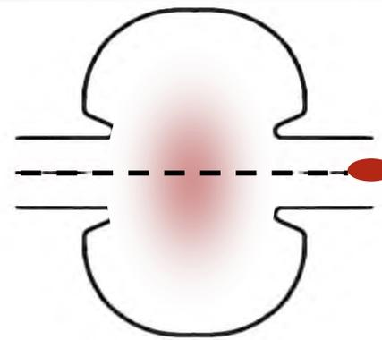
A point charge crosses a cavity initially empty of energy.
