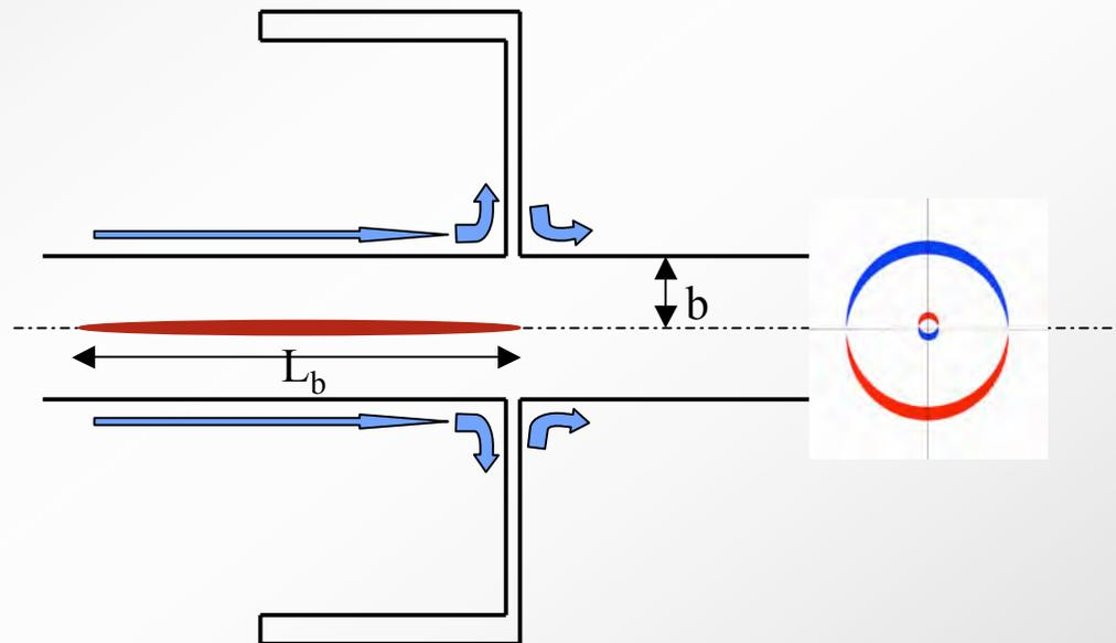
The displacement will grow exponentially even if  $\sigma$  is infinite
