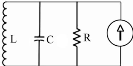
$$Z(\omega) = \frac{R}{1 + jQ \left( \frac{\omega}{\omega_R} - \frac{\omega_R}{\omega} \right)}, \quad \omega_R = \frac{1}{\sqrt{LC}}, \quad Q = R \sqrt{\frac{C}{L}}$$
